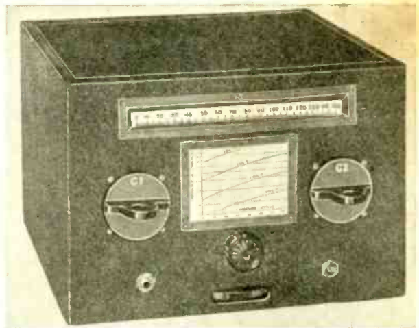
Fig. 2. Front view of the new FB-7 receiver. The full vision scale is marked off in 150 divisions. The tuning calibration curve for each one of the five sets of coils is mounted on the panel. Directly below the tuning control there is the calibrated volume control, of the type which has proven so popular in measuring signal intensity. The coils plug in from the front. Phone jack is located at the lower left-hand corner of the front panel; switch in lower right-hand corner throws the beat frequency oscillator in and out of circuit.
