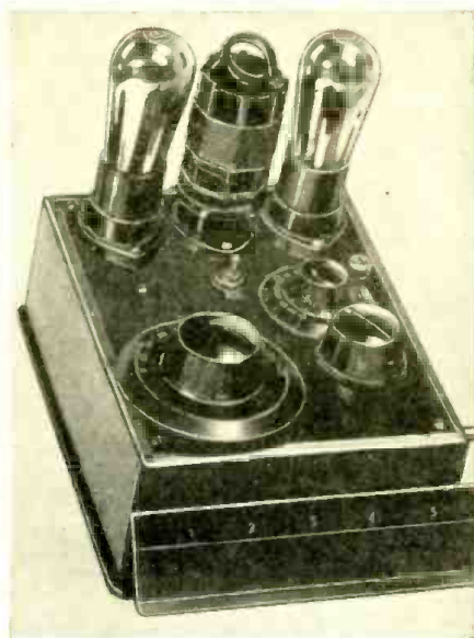
The remarkably clever All-Purpose Receiver here described by Mr. Cullen, who explains how to use this instrument as a wavemeter, monitor, test oscillator, etc.
